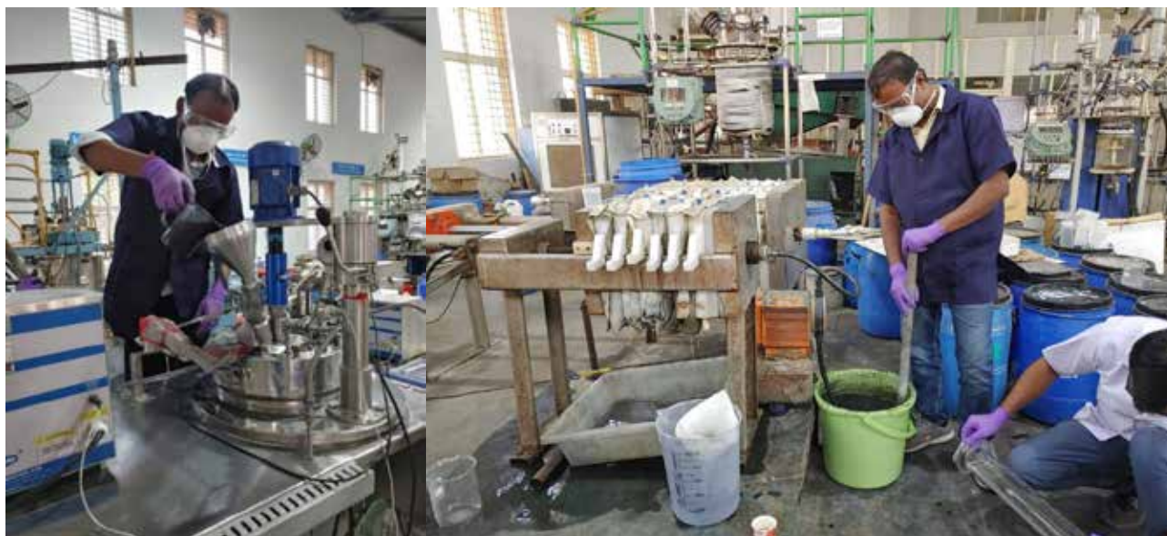
Figure 7: Hydrometallurgical processing of SPL for removal of hazardous constituents
