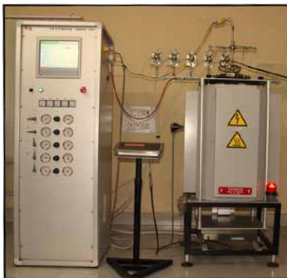
Figure: Multi-standard Test Equipment for Metallurgical testing of iron ore pellet
