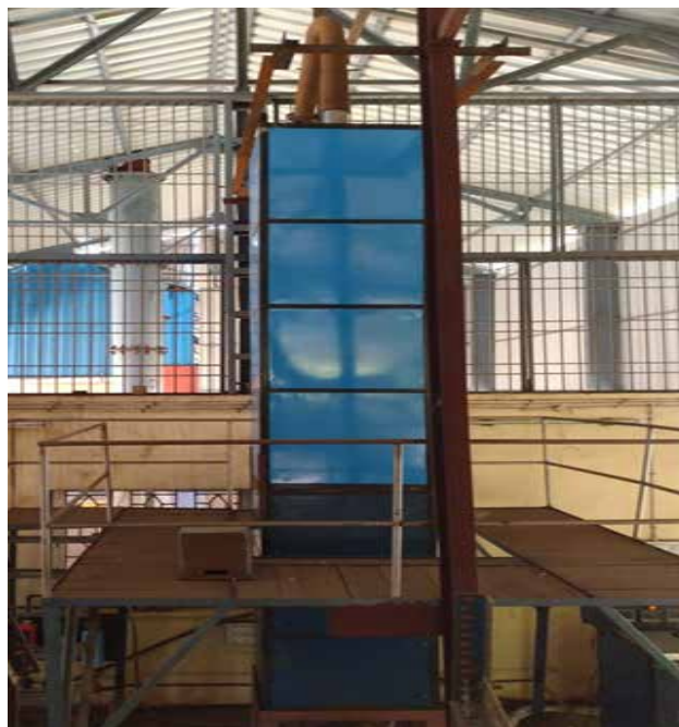
Figure 1: Modified Continuous Fluidized Bed Reactor (100 kg/hr)
