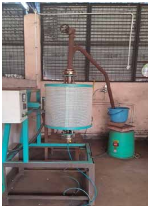
Figure 3: Modified Lab-scale fluidized bed setup with the provision for gas supply
