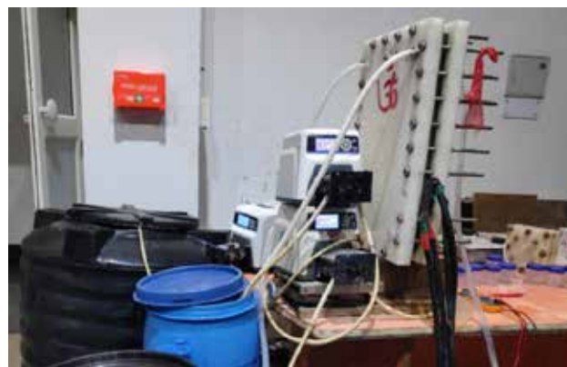
Figure 3: Removal of iron from acidic solution and ammonium sulphate splitting with 1000 cm 2 cell
