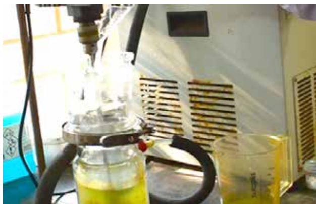
Figure 3: Removal of iron from acidic solution and ammonium sulphate splitting with 1000 cm 2 cell
