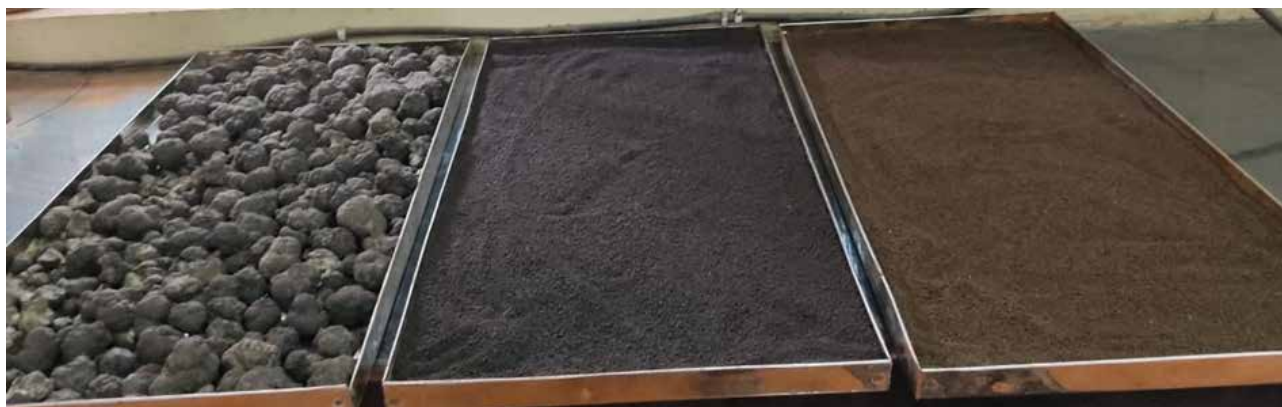
Figure 1: Polymetallic nodules received as such, pelletized nodules and reduced pellets
