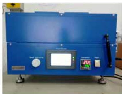
Automatic Film Coater with Vacuum Chuck and Doctor Blade
