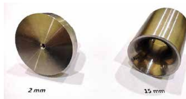
2mm and 15 mm throat diameter CFVN for nozzle bank of the pneumatic conveying setup.
